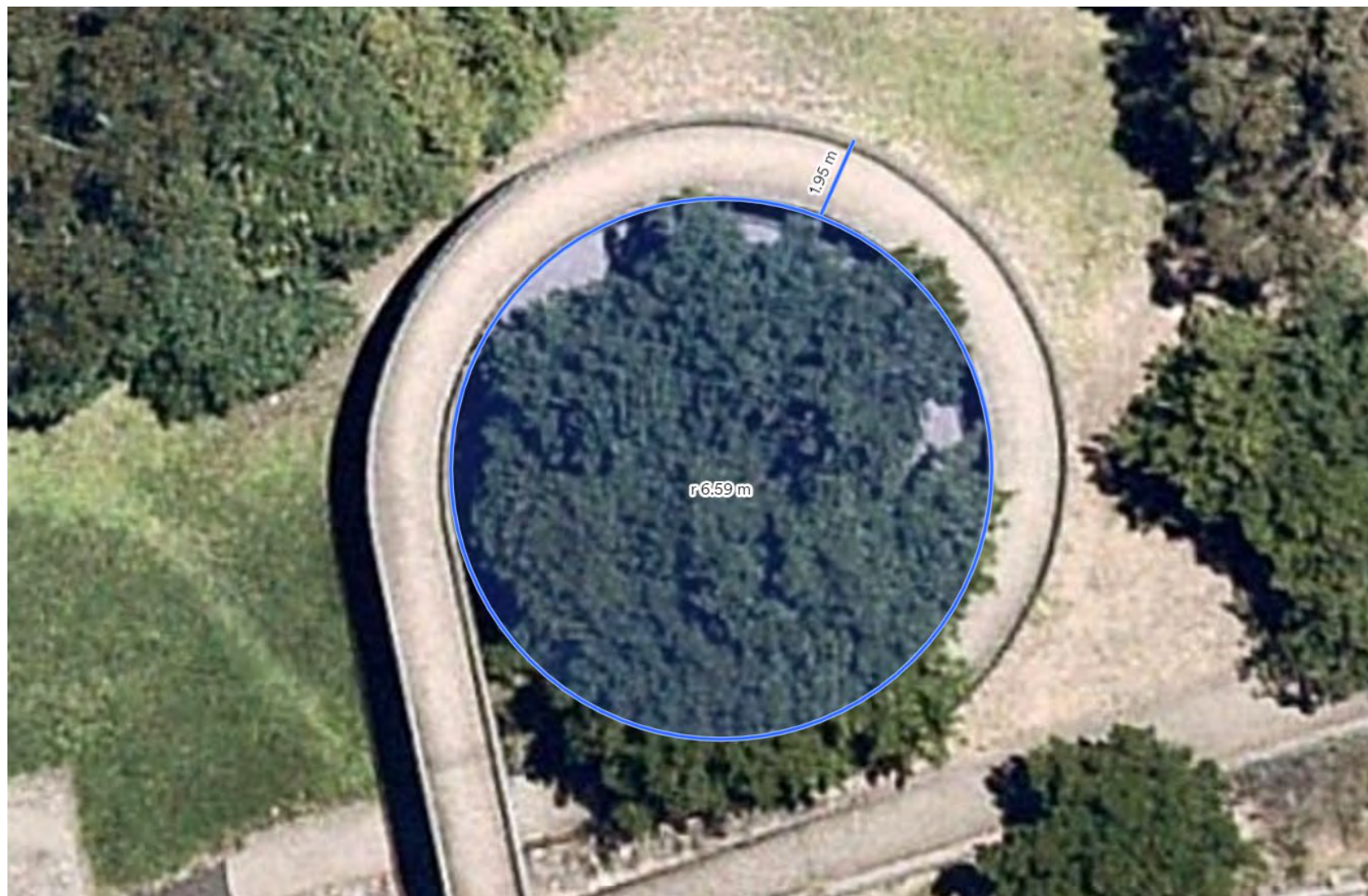
Victoria Road Huntleys Point – inside structure radius – 7.0m approx., width 2.0m approx.
