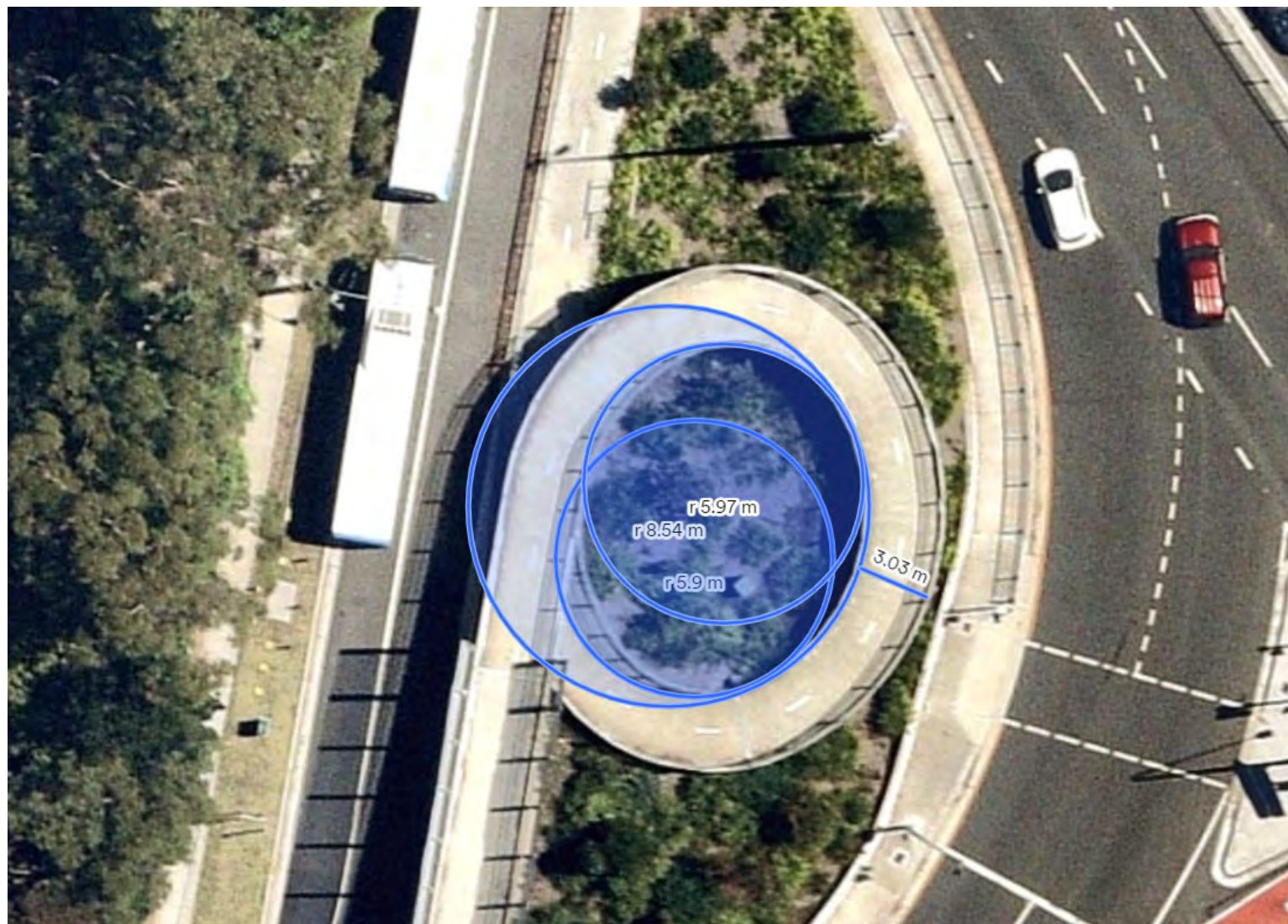
Forest Way Frenchs Forest – Compound Curve Ellipse (inside structure radii – 6.0m & 8.5m approx.) Width 3.0m approx.
